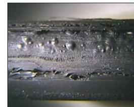
O-ring exposed to rapid depressurization
